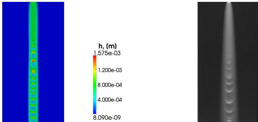
Figure 4: Results of simulation of the rivulet type flow using `REACTINGPARCELFILMFOAM`. The simulated liquid is DC10 silicon oil of  $\gamma = 12 \text{ mN m}^{-1}$  and  $\mu = 10 \text{ mPa.s}$ . Liquid flow rate is equal to  $1.2 \text{ mls}^{-1}$  and plate inclination angle,  $\alpha$ , to  $\pi/4$ . A photo of a rivulet type flow under the same conditions is depicted for reference.
