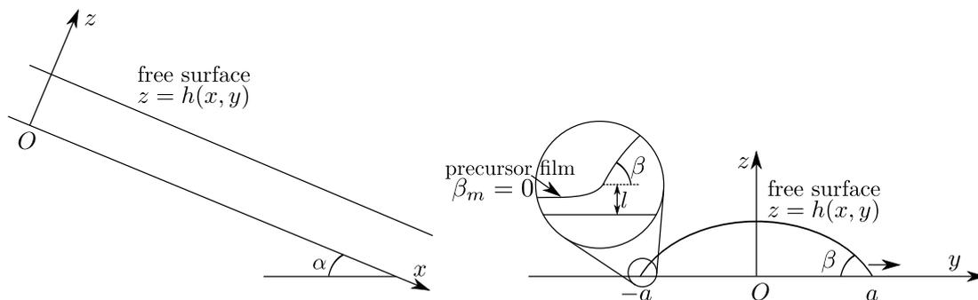
Figure 1: Used coordinate system with the basics of the rivulet spreading notation;  $\alpha$  is the plate inclination angle,  $\beta$  and  $\beta_m$  are the apparent and the microscopic contact angles,  $a$  is the rivulet half width and  $l$  is the problem inner length scale.
