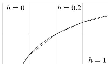
Figure 2: Principle of VOF method. The interface is depicted with a solid line, its geometric reconstruction using piecewise linear function is depicted with a dashed line.
