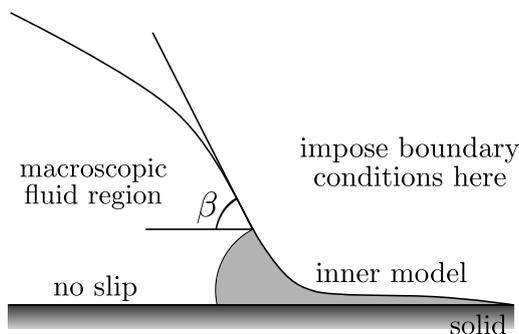
Figure 3: Schematic of procedure for continuum modeling
