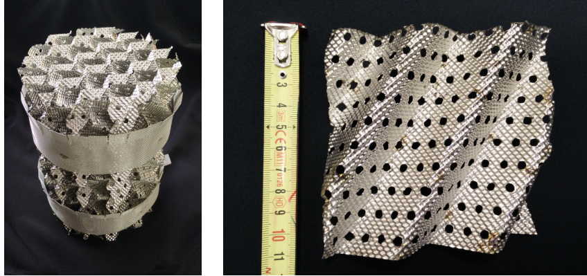
Figure 1: Example of a separation column packing – Mellapak 250.Y. An overall view of the packing is depicted on the left. On the right, there is shown a detail of one element of a dismantled packing. Structured packing usually consists of corrugated, perforated and textured steel plates. Standard mode of operation is counter-current: liquid phase flows down and gas phase up.
